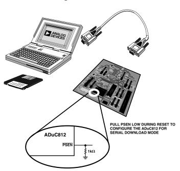
Figure 15. Flash/EE Memory Serial Download Mode Programming
